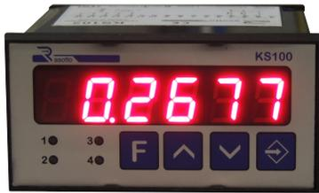
Digital position controller with 5Vdc line driver encoder input. By means of its pulse correction coefficient, the instrument adapts each encoder pulse to the desired measure unit.
